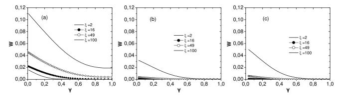
Fig.6: Distributions of mass fraction profiles at different locations for  $q_W = 2000 Wm^{-2}$ ,  $\gamma = 0.01$ , Re = 1000 and  $T_0 = 20^{\circ}C$ .
