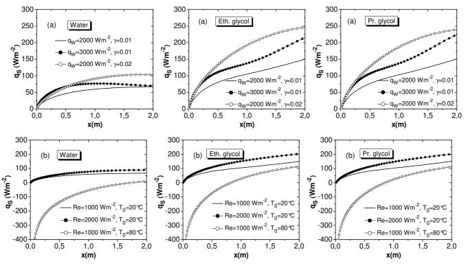
Fig.7: Comparing profiles of sensible heat flux along the channel of Water, Ethylene glycol and Propylene glycol for: (a) Re = 1000,  $T_0 = 20^{\circ}C$ , (b)  $q_w = 2000 Wm^{-2}$ ,  $\gamma = 0.01$ .
