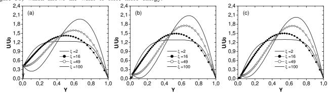
Fig.4: Distributions of axial velocity profiles at different locations for  $q_w = 2000 Wm^{-2}$ ,  $\gamma = 0.01$ , Re = 1000 and  $T_0 = 20^{\circ}C$ .
