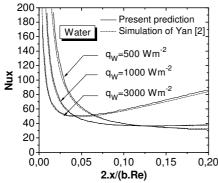
Fig 2.Axial evolution of total Nusselt number Nux for water film for  $B_0 = 0.02 \, kgm^{-1} s^{-1}$ , Re = 1000 and  $T_0 = T_{\ell 0} = 20^{\circ}C$  and  $d = 0.015 \, m$ .
