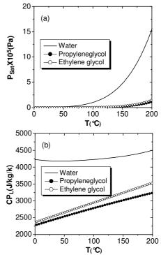
Fig. 3 Evolution of thermophysicals properties of water, propylene glycol and of ethylene glycol with temperature.
