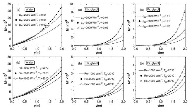
Fig.9: Comparing profiles of dimensionless accumulated mass evaporation rate along the channel of Water, Ethylene glycol and Propylene glycol for: (a) Re = 1000,  $T_0 = 20^{\circ}C$ , (b)  $q_w = 2000 Wm^{-2}$ ,  $\gamma = 0.01$ .
