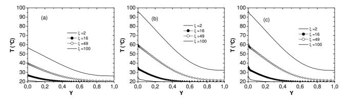
Fig.5: Distributions of temperature profiles at different locations for  $q_w = 2000 Wm^{-2}$ ,  $\gamma = 0.01$ , Re = 1000 and  $T_0 = 20^{\circ}C$ .
